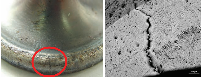
Fig. 12. A crack in a padding weld made on a W-46 engine valve
