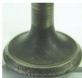
Fig. 3. Erosive wear of a valve face
