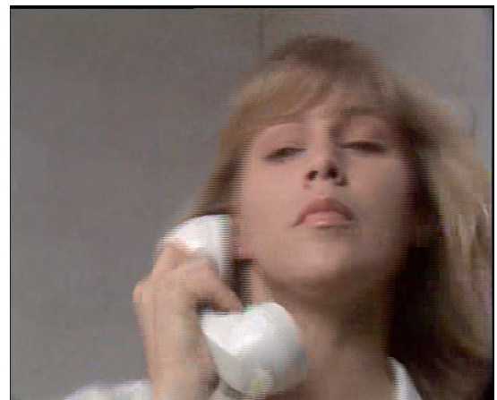
Fig. 4. Compression artifacts in 7 th second of the 'susi' sequence coded with the bitrate of 2 Mbps, blockiness effect appears mainly in the area of hair.
