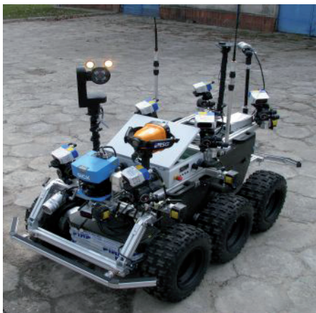
Fig. 1. IBIS robot: a – commercial version with manipulator; b – autonomy research variant.
