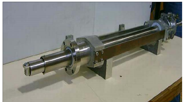
Fig. 22. Picture of a new four-channel Cherenkov-type detector head, designed and manufactured for ISTTOK experiments and installed within the positioning equipment [5].
