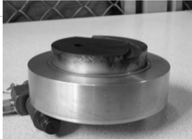
Fig. 4. View on directional groove in lower face of cylinder head
