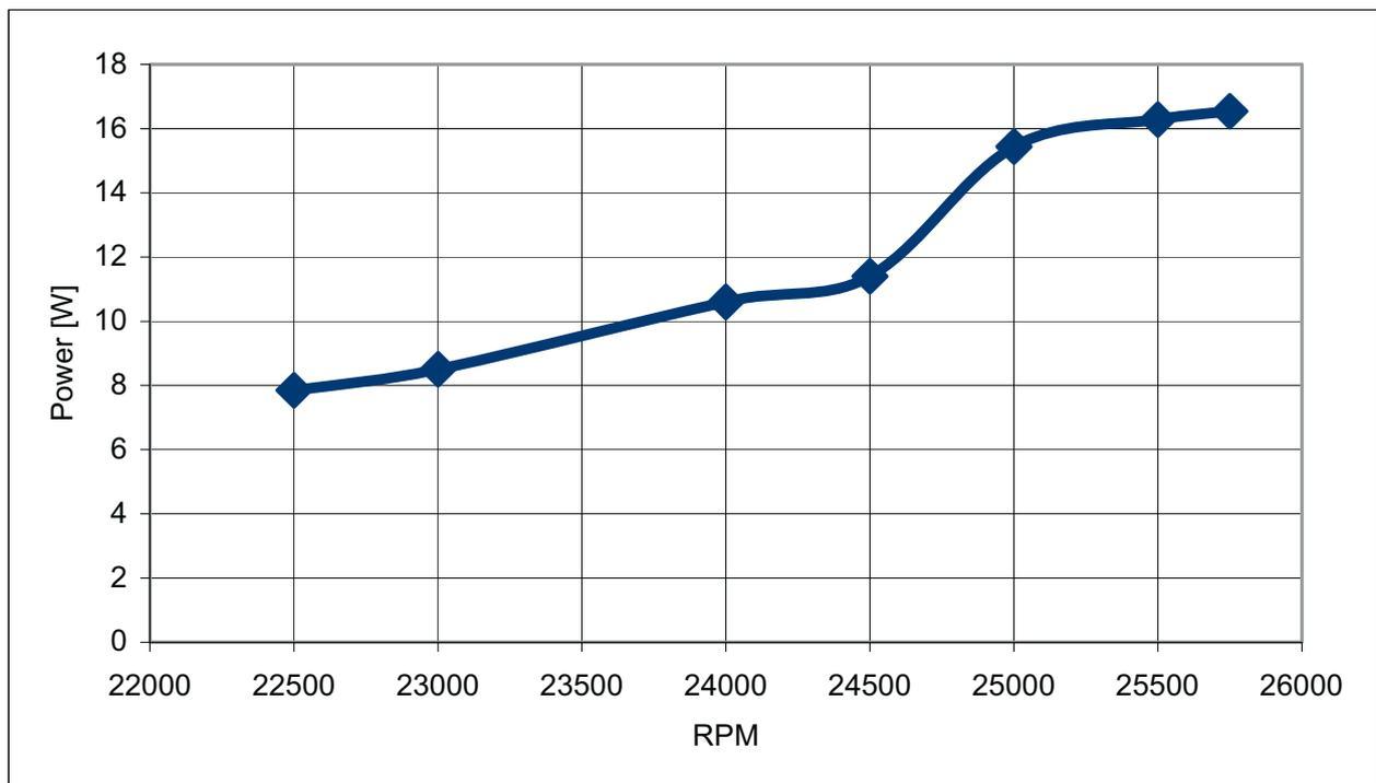
*Fig. 6. The graph of the maximum power for the miniature engine supplied with MN60 fuel*
