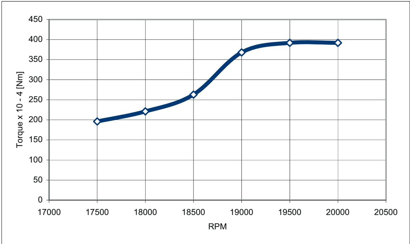
Fig. 7. The graph of output shaft torque for the miniature engine supplied with EN60 fuel
