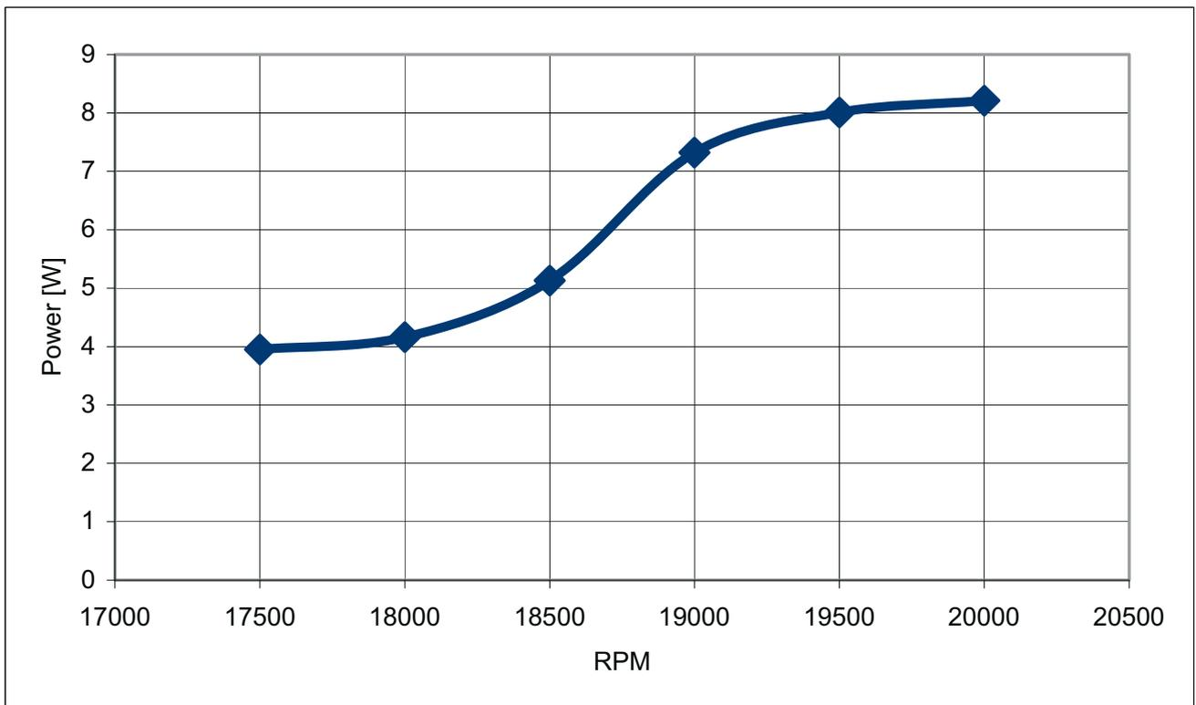
Fig. 8. The graph of the maximum power for the miniature engine supplied with EN60 fuel
