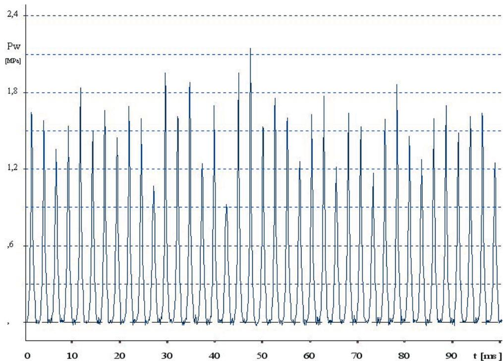
Fig. 4. Exemplary graph of compression pressure in mini combustion chamber on the prototype of a miniature propeller shaft engine supplied with fuel designated by the symbol M80.
