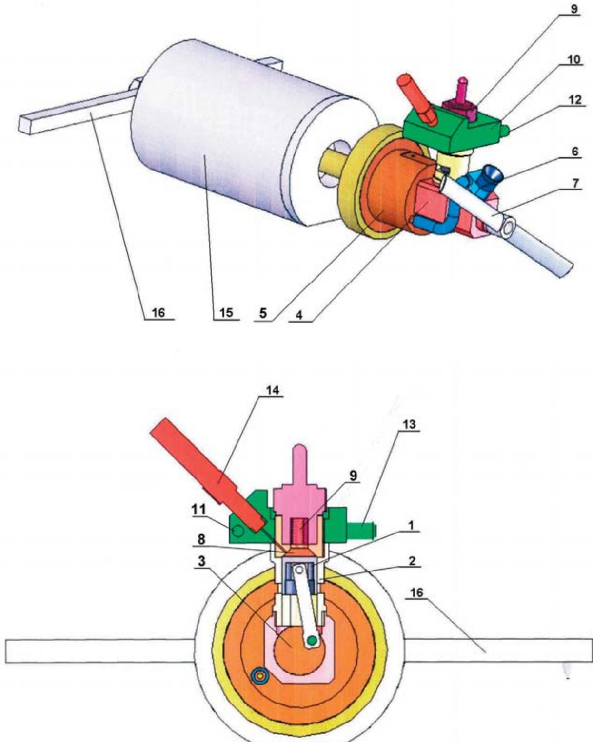
Fig. 1. The view of the miniature propeller shaft engine, together with the miniature brake
