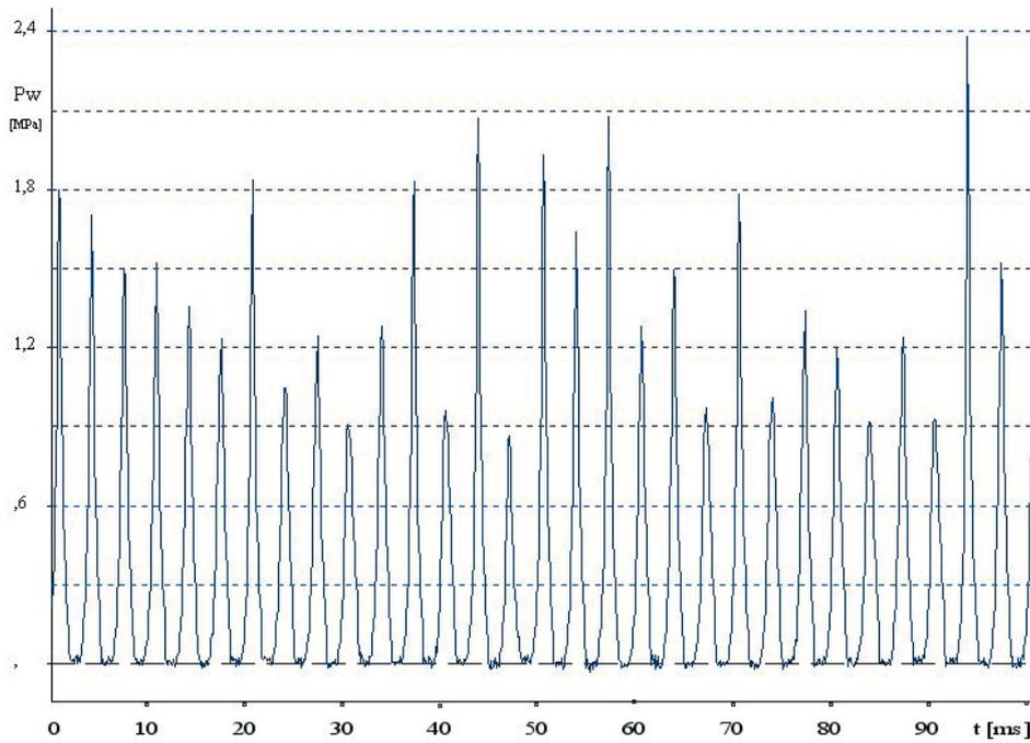
Fig. 3. Exemplary graph of compression pressure in mini combustion chamber on the prototype of a miniature propeller shaft engine supplied with fuel designated by the symbol EN60.
