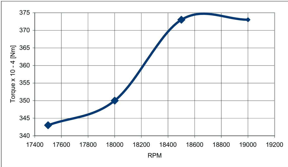
Fig. 9. The graph of output shaft torque for the miniature engine supplied with M80 fuel
