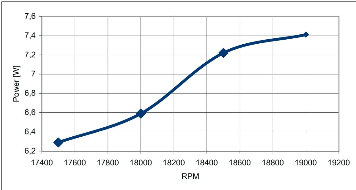
Fig. 10. The graph of the maximum power for the miniature engine supplied with M80 fuel
