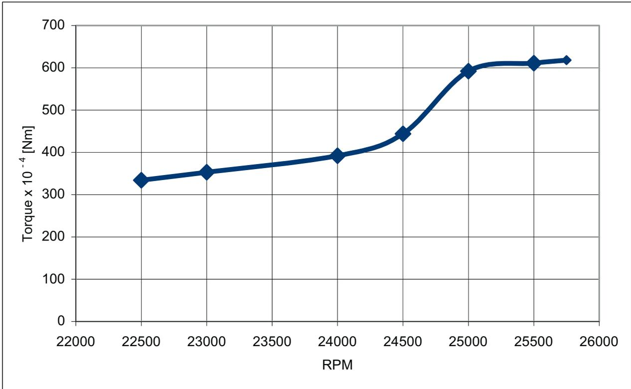
*Fig. 5. The graph of output shaft torque for the miniature engine supplied with MN60 fuel*
