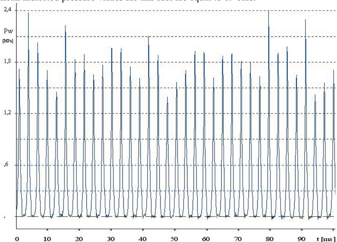
*Fig. 2. Exemplary graph of compression pressure in mini combustion chamber on the prototype of a miniature propeller shaft engine supplied with fuel designated by the symbol MN60.*
