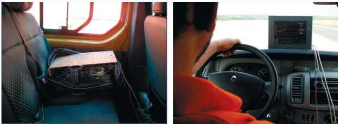
Fig. 1: Portable, on-board monitoring system (left) and drive cycle reproduction (right)
