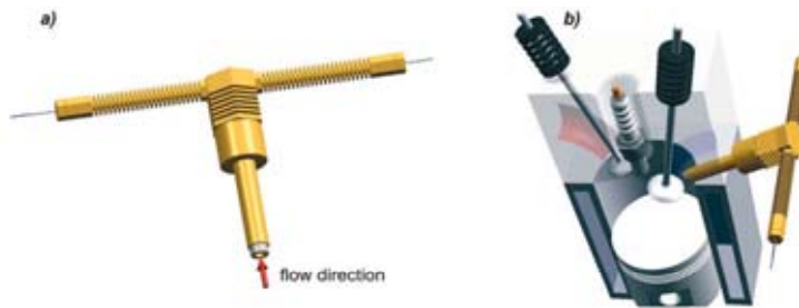
Fig. 2. Measuring head: a - general view, b - measuring head installed in the engine cylinder head
