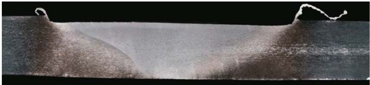
Fig. 5. Cross section of FSW joint No2
