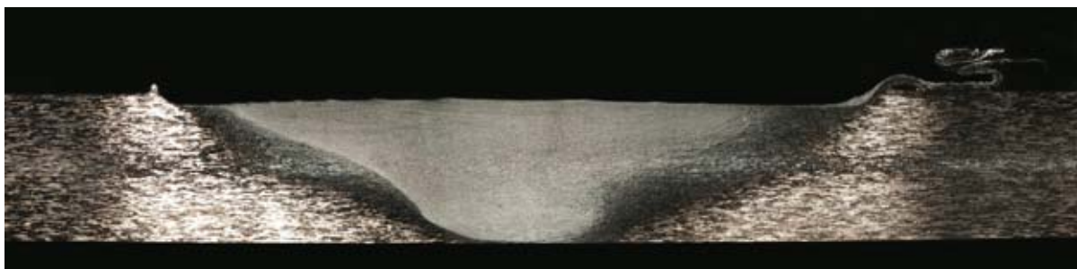
Fig. 7. Cross section of FSW joint No 4
