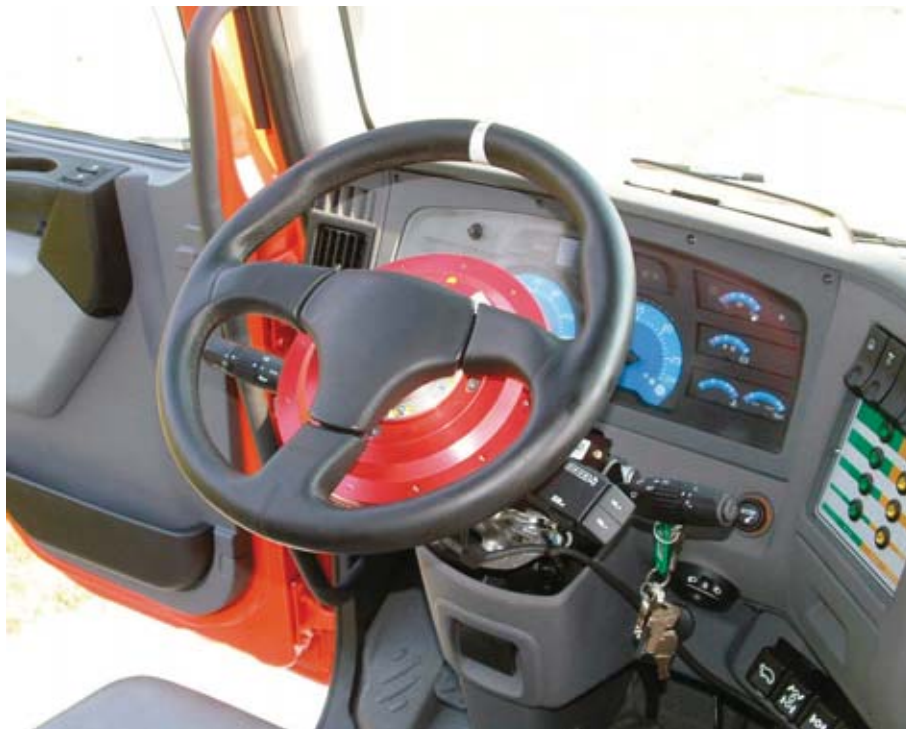
Fig. 6. Measuring steering wheel
