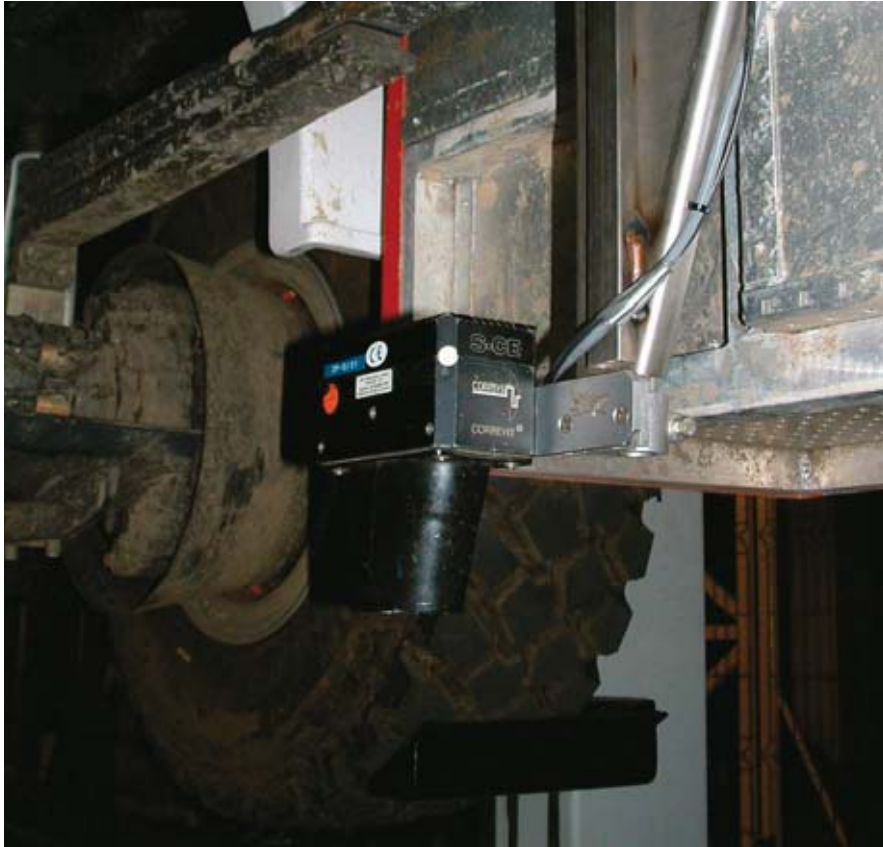
Fig. 7. Attachment of Correvit measuring head under centre of gravity
