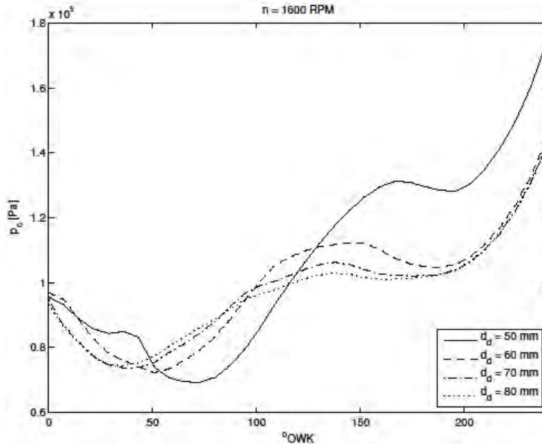
Fig. 1. Dependence of in-cylinder pressure in the function of crankshaft rotation angle at rotational speed of 1600 1/min for different inlet pipe diameters
