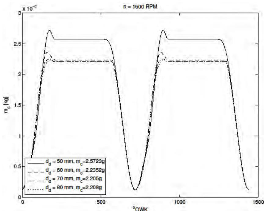
Fig. 3. In-cylinder mass of air in the function of crankshaft rotation angle for the examined inlet pipe diameters at rotational speed of 1600 1/min
