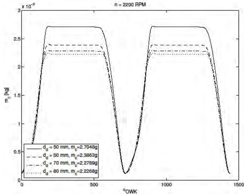
Fig. 4. In-cylinder mass of air in the function of crankshaft rotation angle for the examined inlet pipe diameters at rotational speed of 2200 1/min
