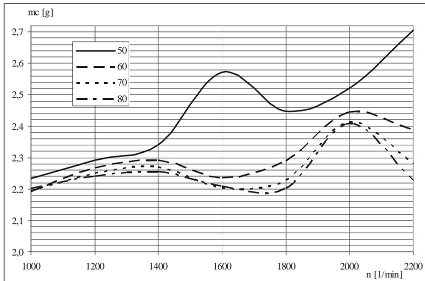
Fig. 5. Dependence of in-cylinder mass on rotational speed at examined inlet pipe diameters
