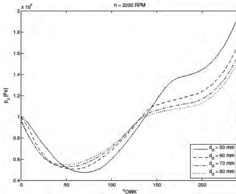
Fig. 2. Dependence of in-cylinder pressure in the function of crankshaft rotation angle at rotational speed of 2200 1/min for different inlet pipe diameters
