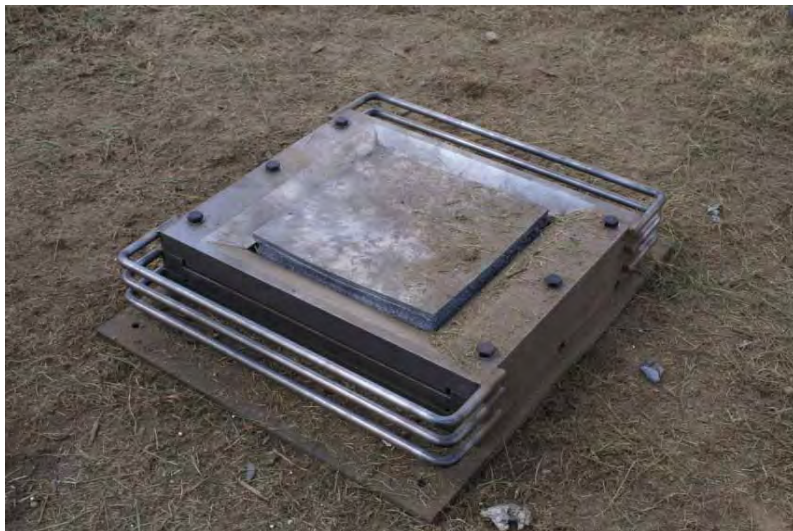
Fig. 6. The SPS system after 2 kg TNT explosion testing
