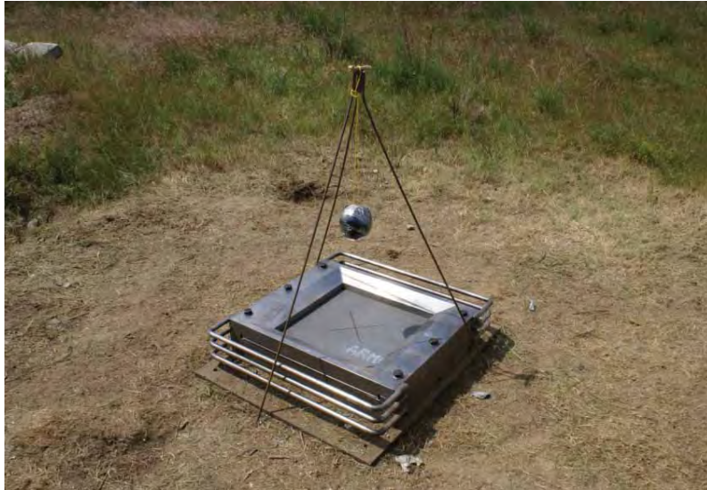
Fig. 2. The PS system before 2 kg TNT explosion testing
