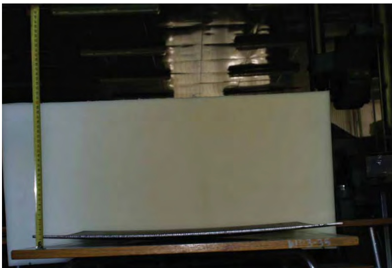
Fig. 4. Plastic deformations of Armox 500T plate removed from the PS system after 2 kg TNT explosion testing
