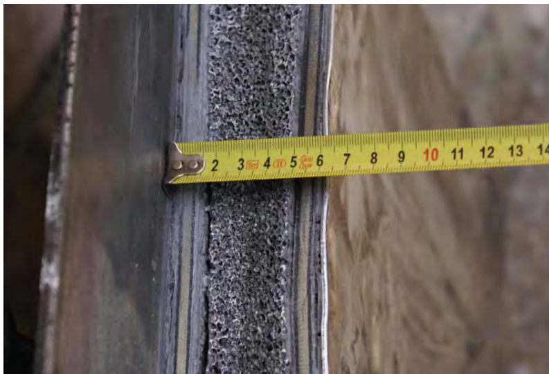
Fig. 7. The exemplary photo of failures in the ALF protective shield removed from the SPS system after 2 kg TNT explosion testing
