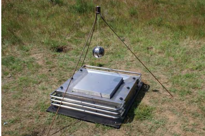
Fig. 5. The SPS system before 2 kg TNT explosion testing
