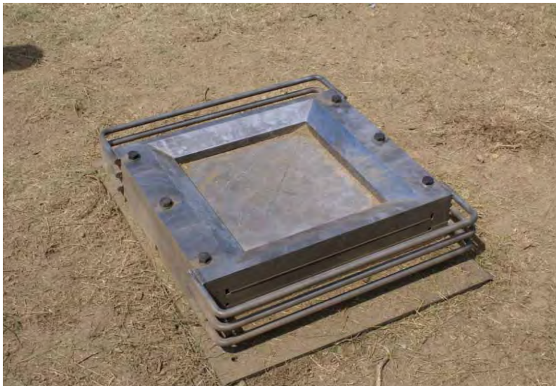
Fig. 3. The PS system after 2 kg TNT explosion testing
