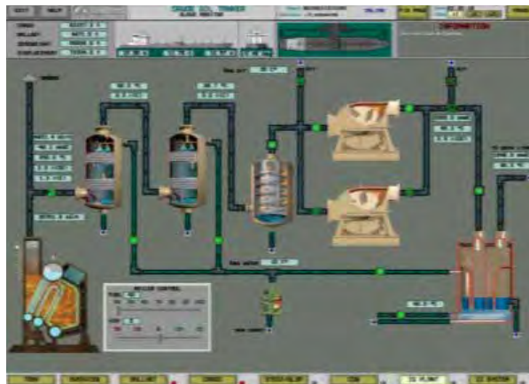
Fig. 7. Loading operations control simulator
