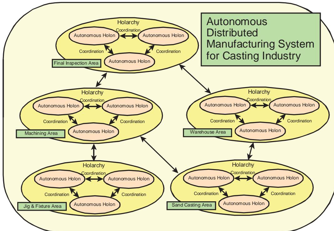
Fig. 3. Model of autonomous distributed manufacturing system for casting industry
