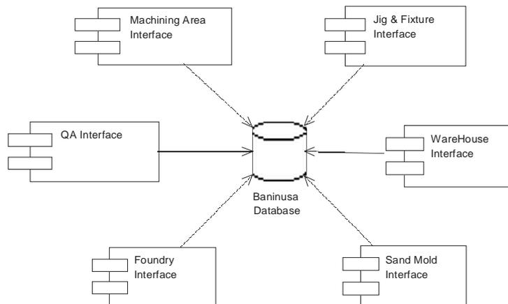
Fig. 10. Component diagram of units in casting industry
