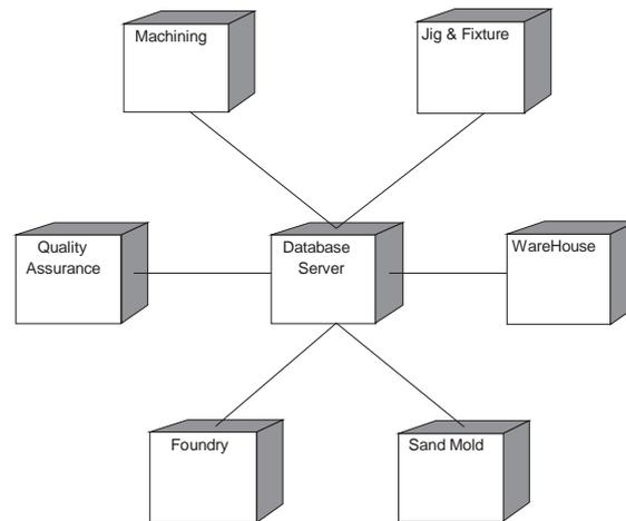
Fig. 11. Deployment Diagram of Hardware at Units that will be Connected with Database Server
