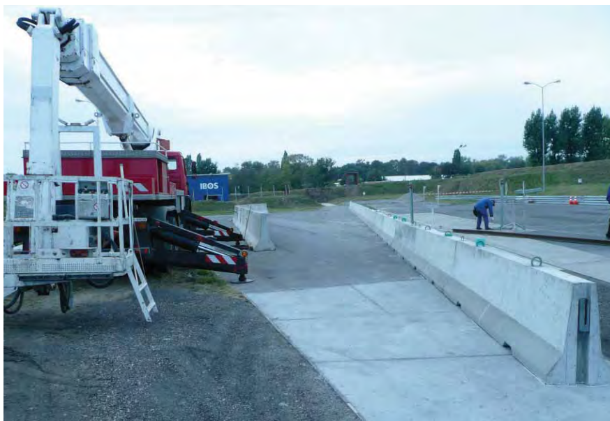
Fig. 1. Prototype concrete barrier placed on the test track in IBSO in Inowrocław, Poland, ready for crash tests
