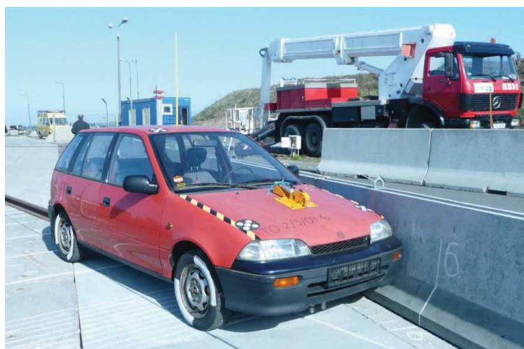
Fig. 2. SUZUKI SWIFT 1.3GL test car prepared for the crash test – car no. I at the crash point
