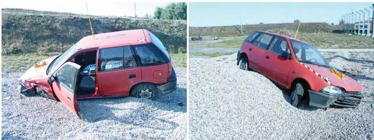
Fig. 6. The test car no. 1 Suzuki Swift 1.3GL after the crash test shown from the driver side and the passenger side
