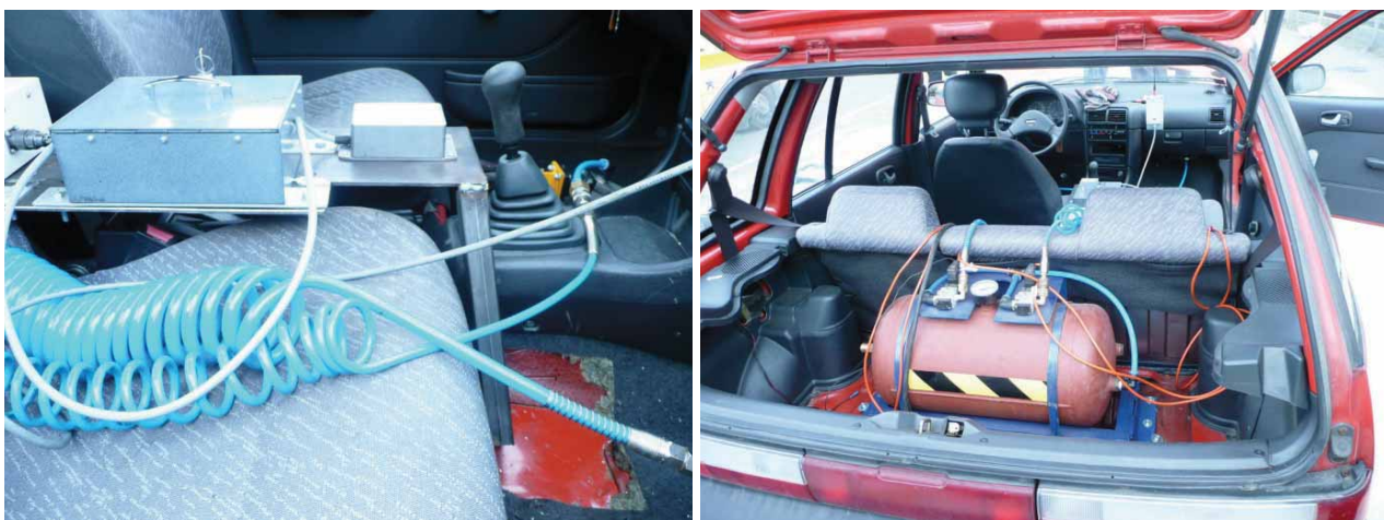
Fig. 3. Arrangement of the ACCINO 2 and 3 measuring systems and control system components in the test car no. I Suzuki Swift 1.3GL
