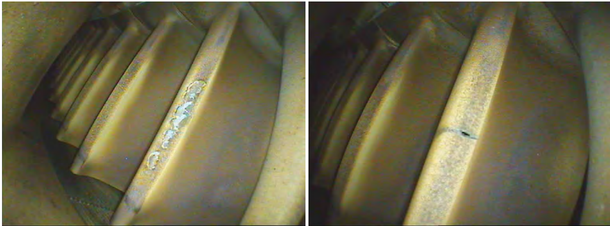
Fig. 1. Temperature-attributable damages to edges of attack of turbine rotor blades, exemplary videoscope records [1]
