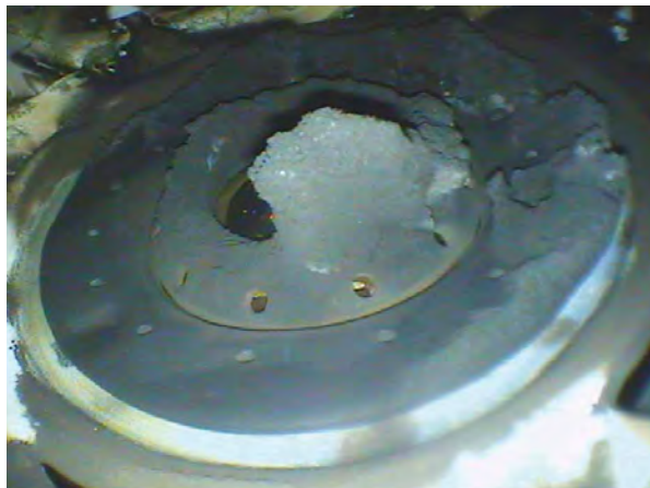
Fig. 3. Carbon deposit on the fuel injector in the gas turbine engine [2]
