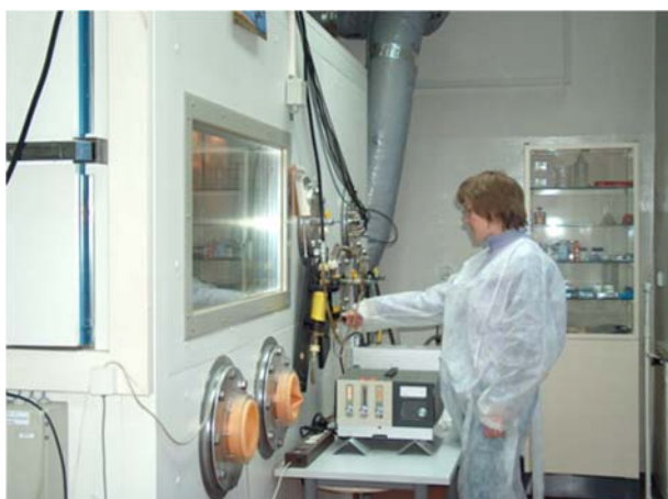
Fig. 1. The walk-in radon calibration chamber of CLOR.
