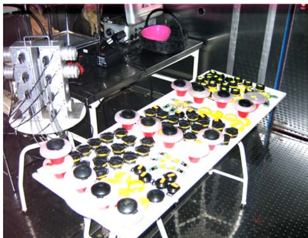
Fig. 4. Exposition of diffusion chambers with CR-39 being compared in the radon chamber.
