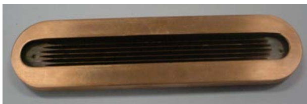
Fig. 2. Grooved copper backing of the molybdenum target proved to enhance cooling during irradiation (back surface of the molybdenum target).
