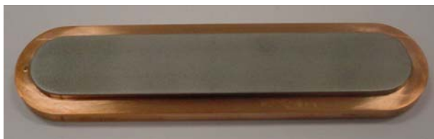
Fig. 1. Natural molybdenum coated as a metallic layer on copper backing (front surface of the molybdenum target).
