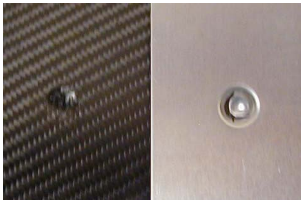
Fig. 13. 4 ply X-ray cured carbon fiber composite and aluminum panel of the same thickness impacted at 13.6 N-m.
