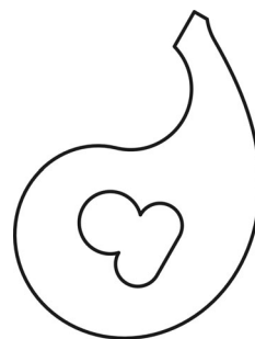
(b) CAD drawing of cam
