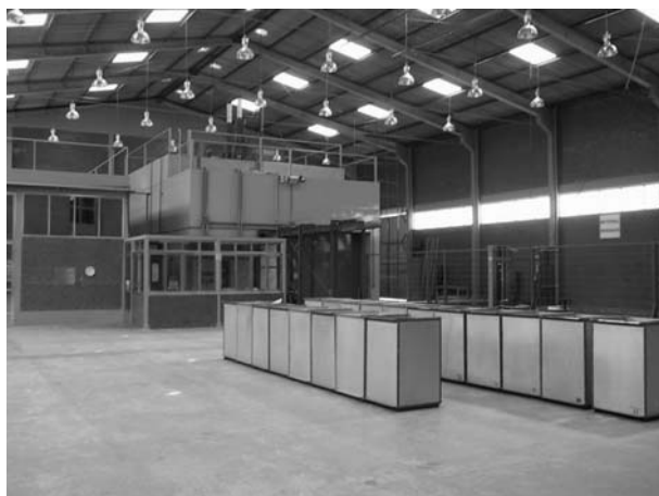
Fig. 3. Compact type cobalt-60 multipurpose irradiator, projected, constructed and implanted in the IPEN-CNEN/SP, by a national technology and FAPESP financial support.
