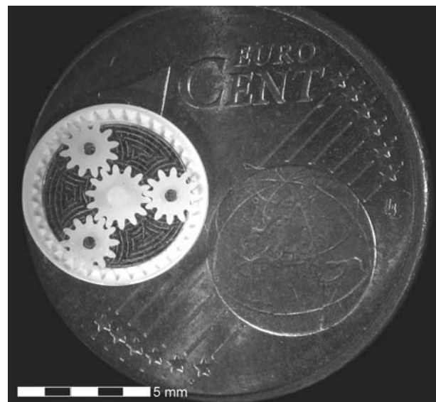
Figure 3. Micro planetary gear on a Cent coin.
