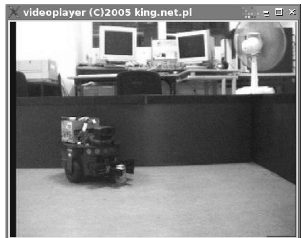
Fig. 12. The same situation as in figure 11 seen by the robot's camera (it cannot see 180 degrees as laser do, so this image shows less information about obstacles than laser scans presented earlier).
