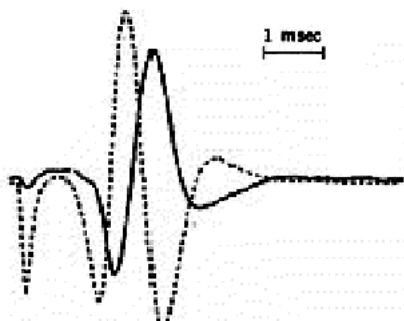
Fig. 3. The magnetic (solid lines) and electric (dashed lines) signals recorded from a frog sciatic nerve immersed in Ringer solution.
