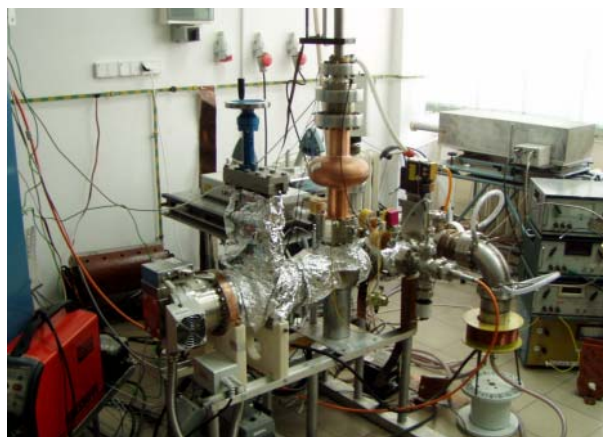
Fig. 17. UHV stand equipped with the linear (cylindrical) arc plasma source and laser trigger system, built in the frame of the European Community-Research Infrastructure Activity under the FP6 "Structuring of the European Research Area" program (CARE, contract number RII3-CT-2003-506395).
