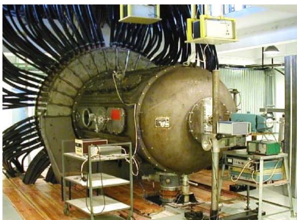
Fig. 6. Experimental chamber of the mega-joule PF-1000 facility, which was designed at IPJ at Świerk, Poland, and assembled at the IPPLM in Warsaw. It is now used by the International Centre for Dense Magnetized Plasma operated under UNESCO auspices.
