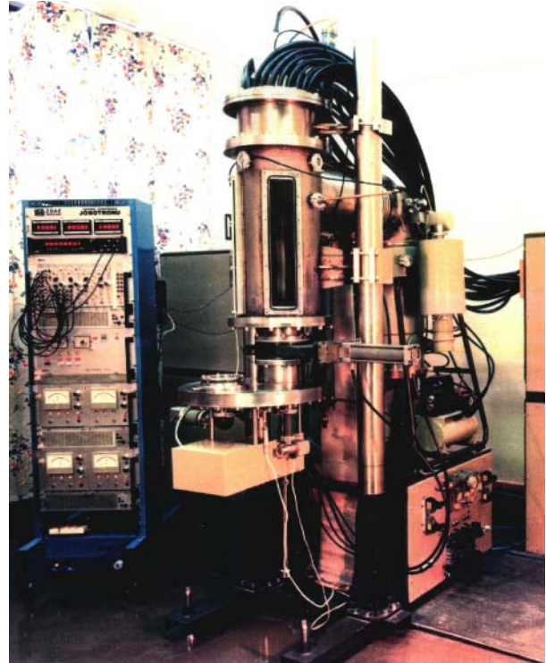
Fig. 15. General view of the IONOTRON-SW30 machine equipped with the RPI-type plasma accelerator of the vertical axis and a carousel holder of samples (below), capacitor banks (behind and on the right), and an electronic control unit (on the left).
