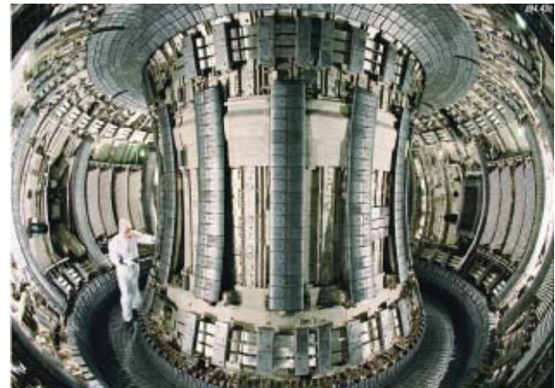
Fig. 2. Large experimental chamber of the JET (Joint European Tokamak) facility. There are shown the central column (containing a yoke of the large transformer used for inducing the main discharge current), some equipment (microwave antennas) for additional plasma heating, diagnostic ports upon the external wall and the divertor region (at the bottom).
