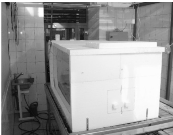
Fig. 1. The expanded polystyrene chamber constructed inside the greenhouse to maintain high humidity necessary for the development of fruitbodies.
