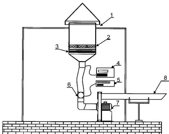
**Fig. 1.** Schematic picture of AZA-1000 set-up. 1 – Suction head cover with air inlet; 2 – 4 infrared heaters; 3 – filter frame tray; 4 – electric box for power supply; 5 – flowmeter display; 6 – flowmeter type VR-600; 7 – air pump high-pressure fan type ZWP-1300 (Venture Industries); 8 – outlet tube.
