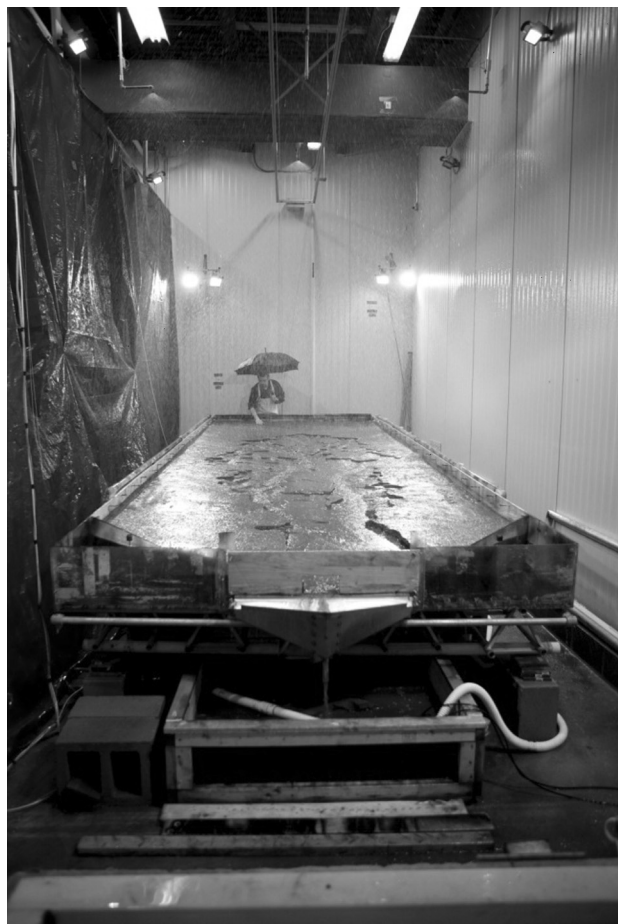
Fig. 1. Experimental landscape facility, University at Buffalo showing rainfall nozzles, camera track, flume and soil bed, and sample collection weir. Flume is 7.0 m long and 2.4 m wide, and flow is from top to bottom
