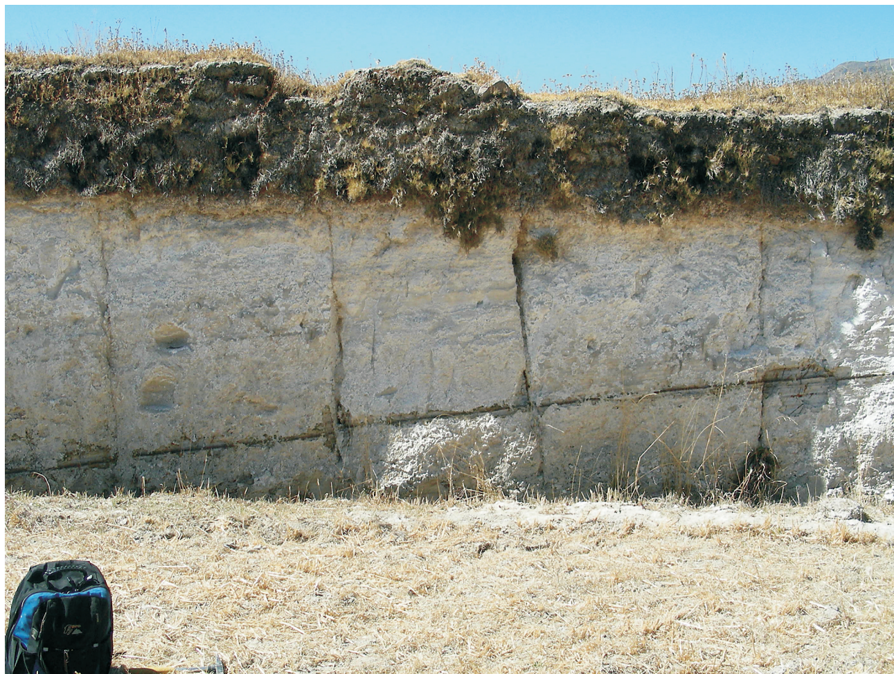
Ryc. 8. Spękania osadów jeziornych w osuwisku Maca Fig. 8. Joints in lacustrine sediments in a landslide at Maca
