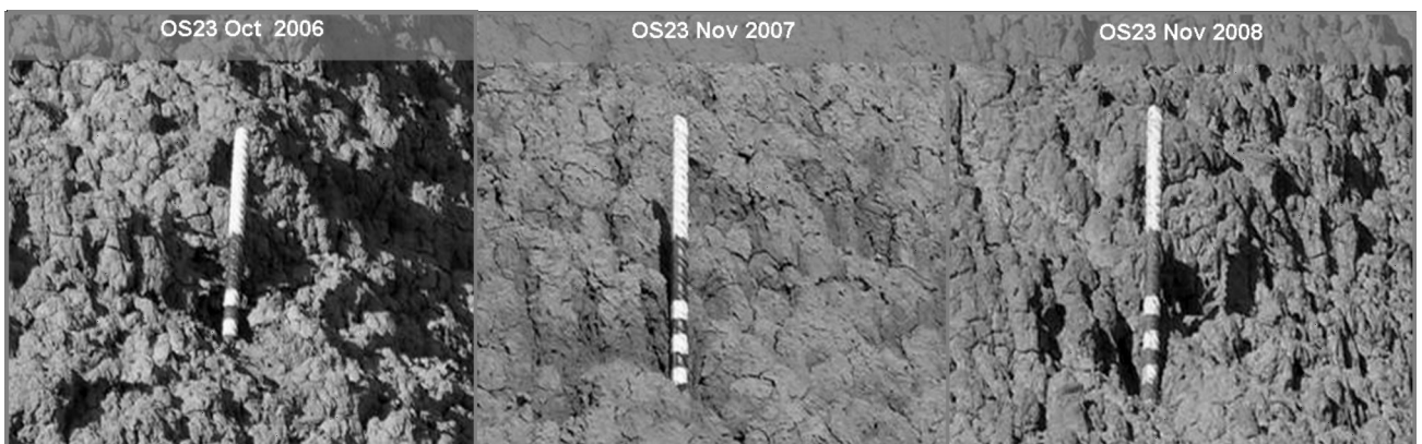
Fig. 4. Ottosalme area: examples of relative height variations of erosion pin
