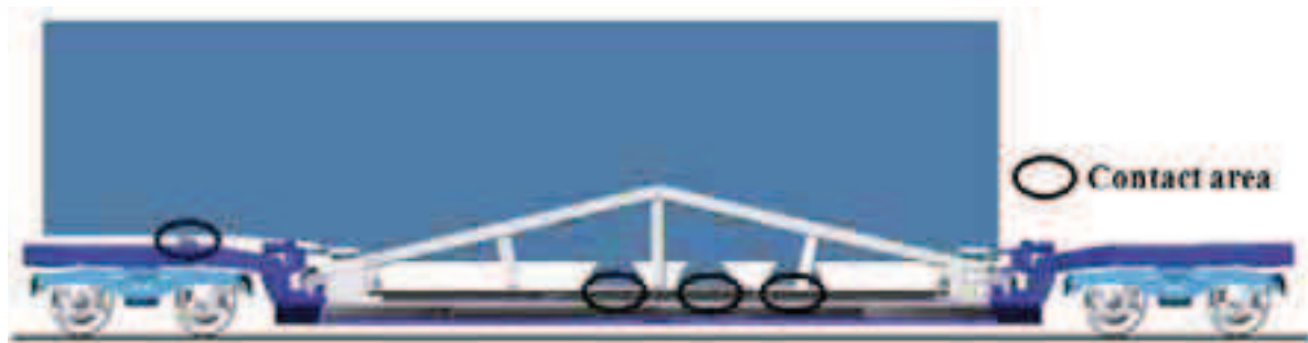
Fig. 6. Constraints mapping fixing of the semitrailer in the saddle and additional contact areas of semitrailer wheels with wagon model
