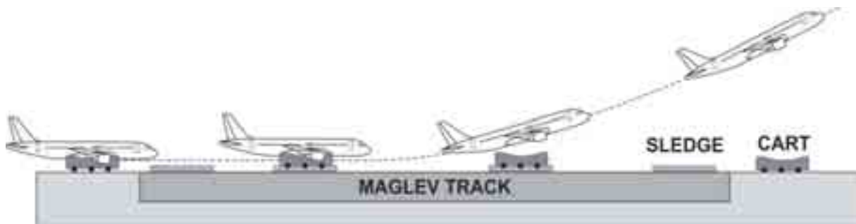
Fig. 4. GABRIEL concept - aircraft carried on the cart and connected to the sledge [7]
