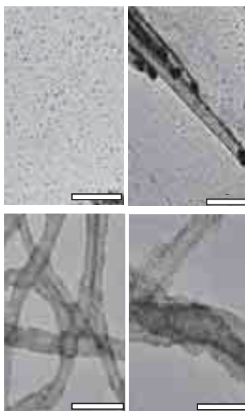
Fig. 1. Pictures from a transmission electron microscope presenting CNTs with the embedded platinum nanoparticles on them
