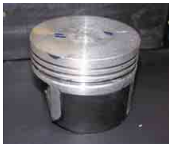
Fig. 4. The piston selected for testing when its side surface is coated with a layer of nanotubes
