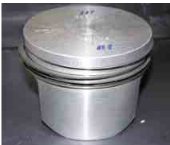
Fig. 3. The piston selected for testing before it is coated with a layer of nanotubes
