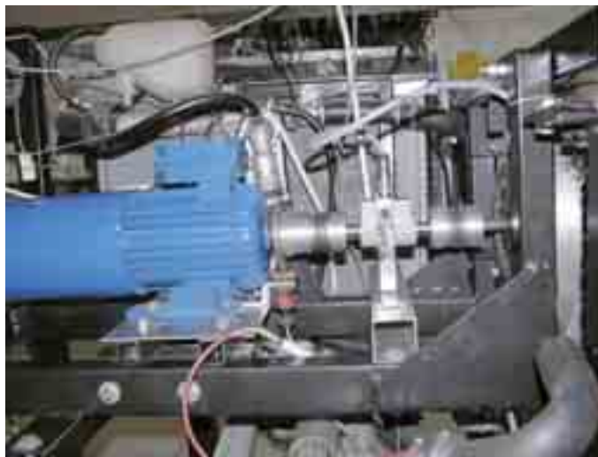
Fig. 9. General view on the test station for measuring the moment of coupling the internal combustion engine with the asynchronous electric motor that drives it
