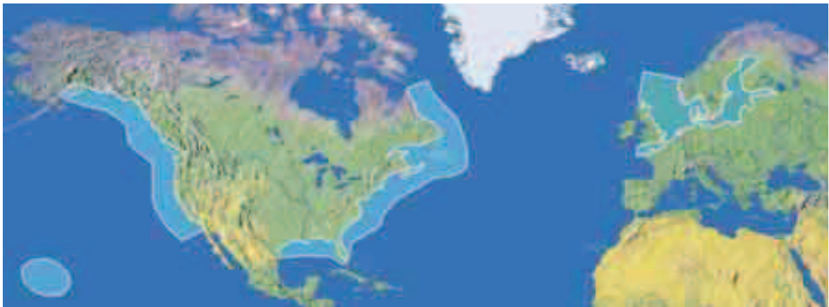
Fig. 1. IMO and EPA emission controlled areas [1]
