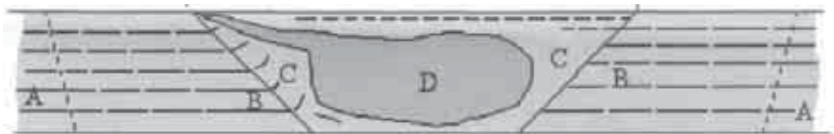
Fig. 1. Schematic diagram of the FSW joint structure welded on one side [P1]
