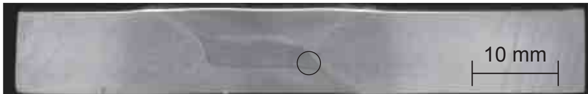
Fig. 2. Macrostructure of FSW welded joint (double-sided welding) - marked by circle welds fragment selected for microscopic examination
