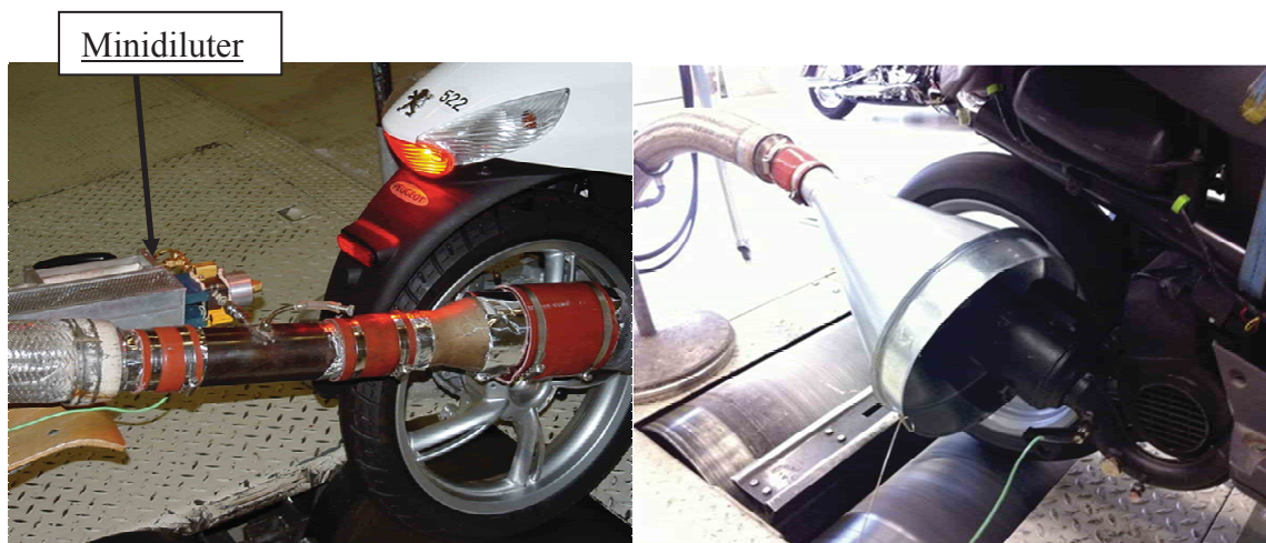
Fig. 1. Passage of exhaust gas from tailpipe to CVS: closed (left), open (right)
