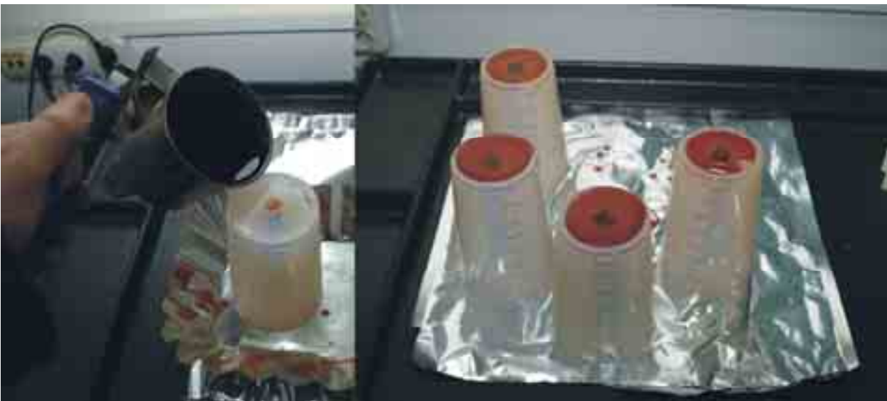
Fig. 5. Silicone mould pouring cylinder core wax model
