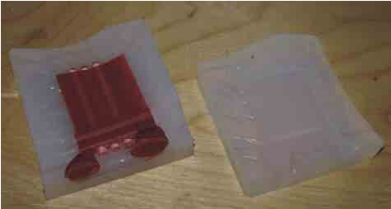
Fig. 4. Wax model of core blade and silicone mould
