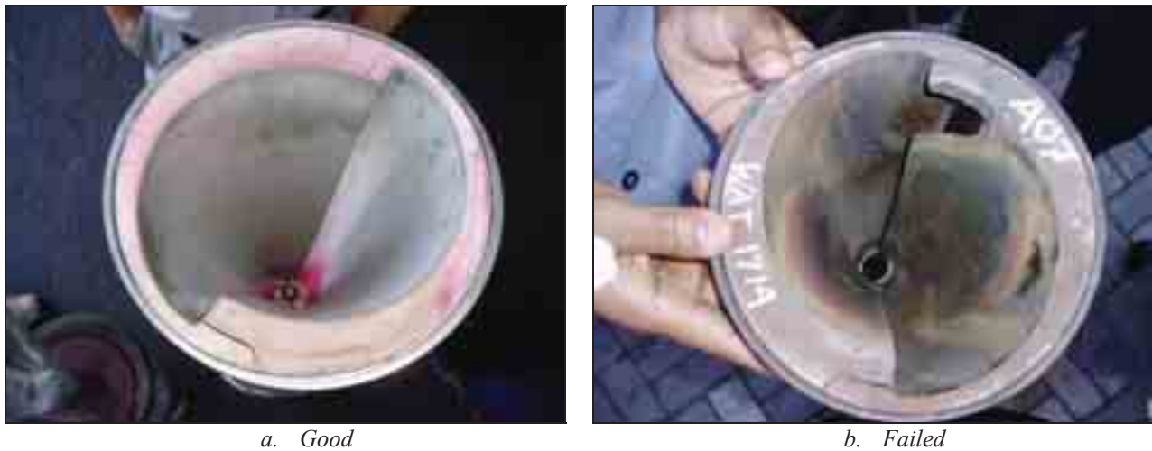
Fig. 2. Comparison between good and failed cone burners
