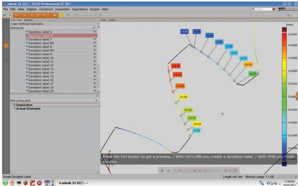
Fig. 7. Detailed analysis of the deviations from the outline of the selected values of the teeth measured wheel
