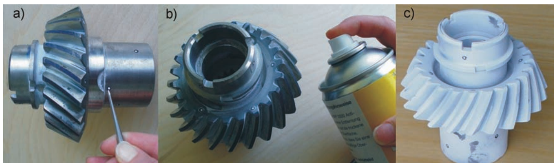
Fig. 2. Preparation of an object to measure: a) affixing markers, b), c) anti-reflective cover
