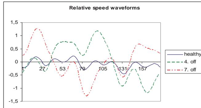
Fig. 4. Comparison of relative angular speed waveforms
