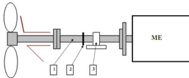
Fig. 1. Layout of ships propulsion with toothed rings mounted at intermediate shaft. 1 – intermediate shaft; 2- measurement toothed rings; 3 – shaft bearing; ME – main engine
