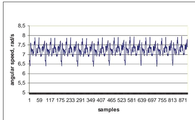
Fig. 2. Wave-form of angular speed fluctuation, 7 healthy cylinders, 10 revolutions recorded
