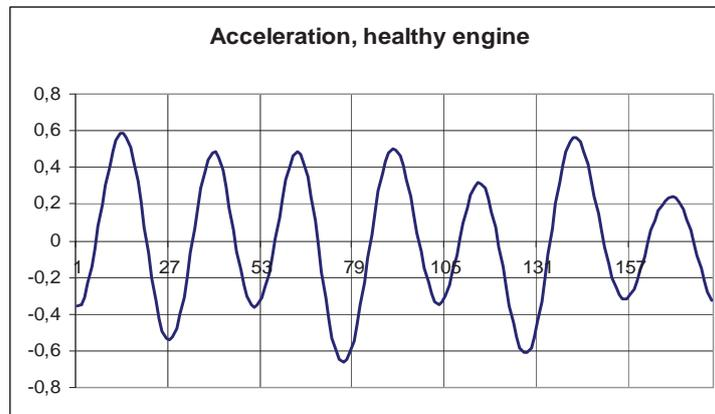
Fig. 8. Angular acceleration of normal working engine, samples of one revolution
