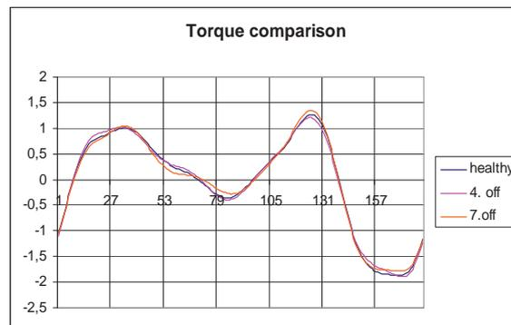
Fig. 5. Comparison of torque run of healthy and misfiring states
