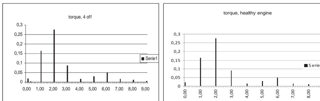
Fig. 6. Spectral analysis of torque course, 4.cyl. off and healthy eng. Domain of frequency (1/eng. cycle)
