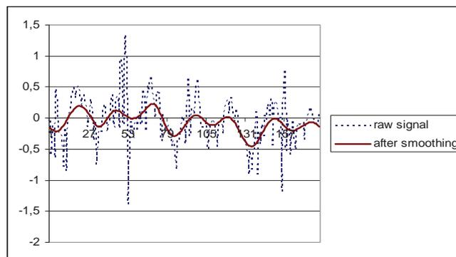
Fig. 3. Recorded angular speed waveform (dotted line) and the same after third step of smoothing. All healthy cylinders, one revolution samples
