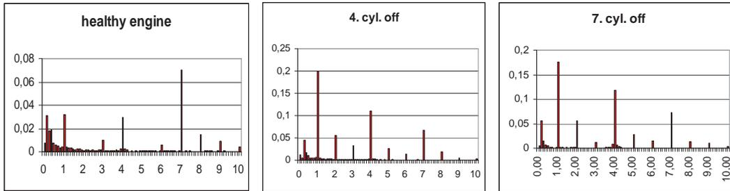
Fig. 7. Spectral analysis of angular speed in domain of frequency (1/eng. cycle)
