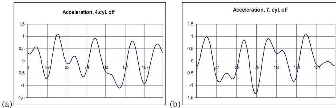
Fig. 9. Deviation of angular instantaneous acceleration (misfiring in cyl.4. and 7)
