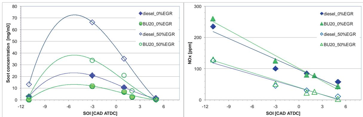
Fig. 3 – Engine exhaust emissions of soot (left) and NOx (right) vs. the start of injection (SOI)
