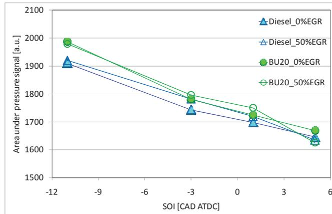
Fig. 2 - Pressure working area vs. the start of injection (SOI) for all the operating conditions
