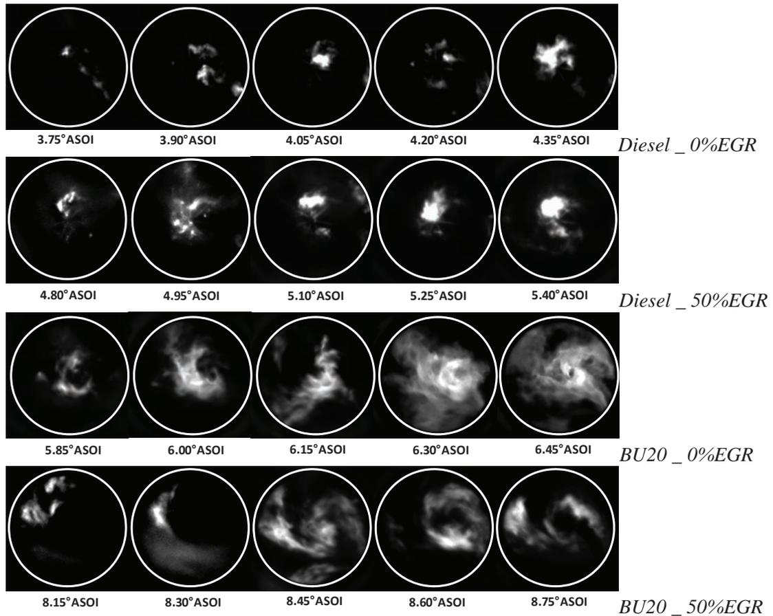
Fig. 7. UV-VIS flame emission for Diesel and BU20 fuel, SOI=5 CAD ATDC (0-50%EGR)
