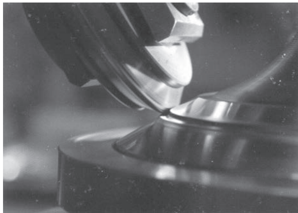
Fig. 1. High pressure on the welded (Nimonic 80A) spindle seat of MAN BW Diesel engines [3]
