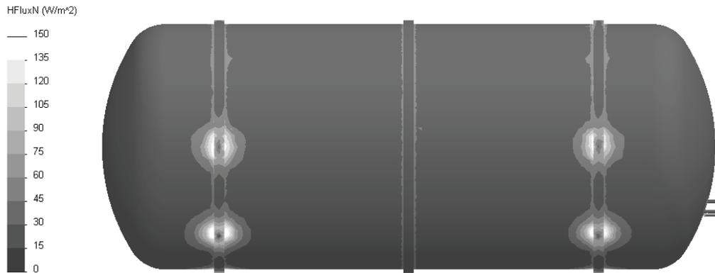
Fig. 4. Heat flux on outer surface of simplified container tank type II
