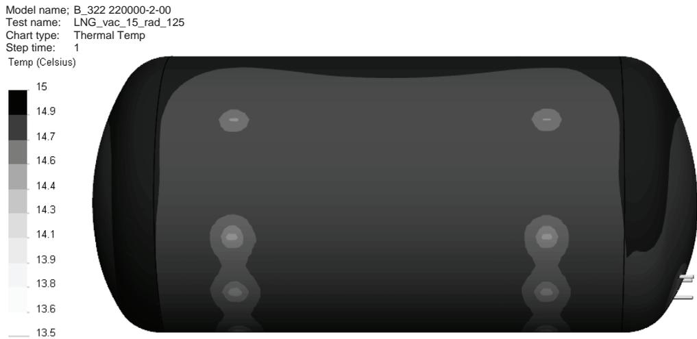
Fig. 8. Temperature distribution on outer surface of stationery tank type IV
