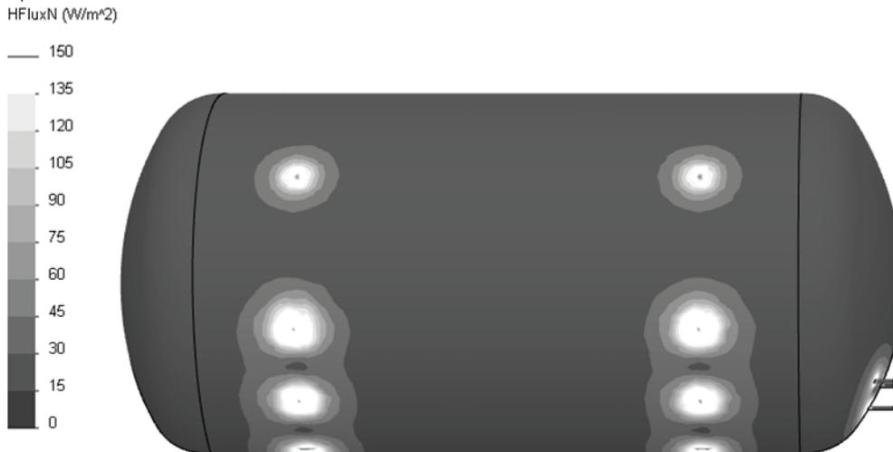
Fig. 5. Heat flux on outer surface of stationery tank type III
