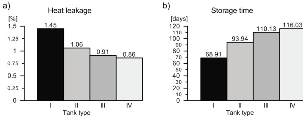
Fig. 10. Comparison of the heat leakages (a) and storage time in days (b) of considered tank versions
