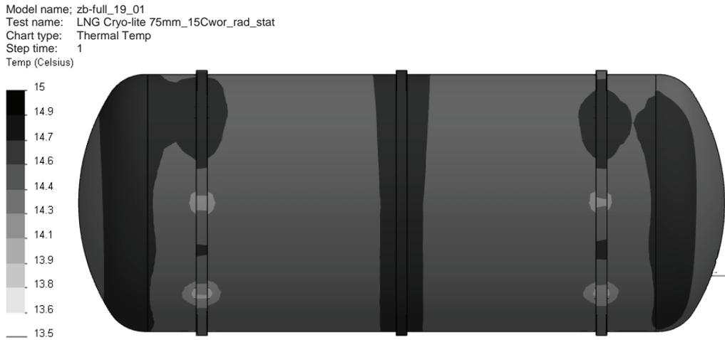
Fig. 7. Temperature distribution on outer surface of stationery tank type II
