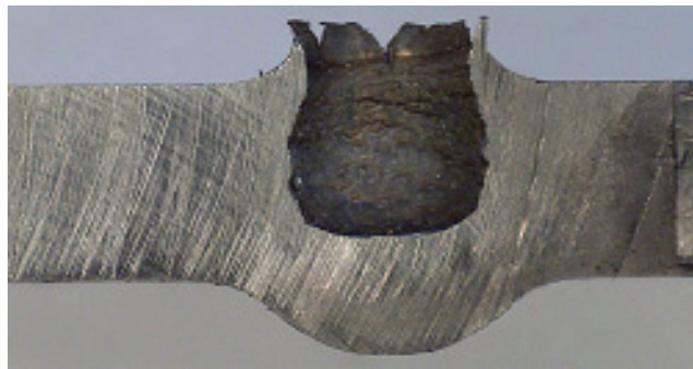
Fig. 1. Macroscopic images of a crater filled with the remains of grinded and eroded rifle missile with traces of adiabatic shear in the cut of steel disc
