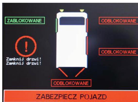
Fig. 3 Touch panel steering the cash transport vehicle
