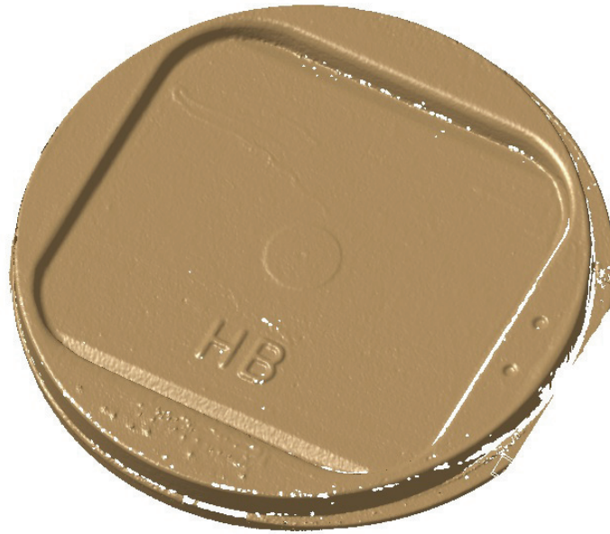
Fig. 1. Surface of the piston crown created by 3D scanning
