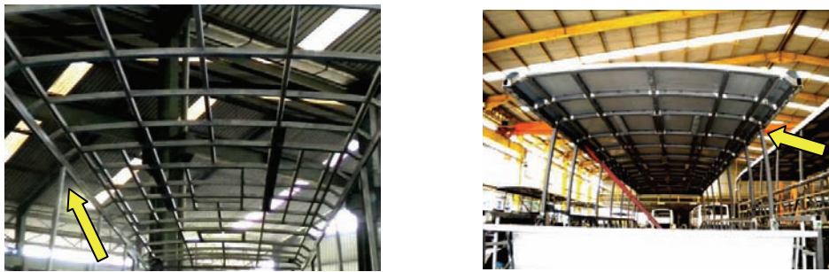
Fig. 3. Pillar and roof bow joint details from two different manufacturers
