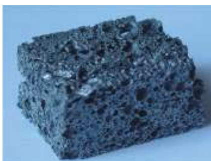
Rys. 1. Badane materiały: a) AK9/SiC z małymi pęcherzami, b) AK9/SiC, c) spieniane aluminium TiH 2 Fig. 1. Tested materials: a) AK9 / SiC in the form of small blisters, b) AK9 / SiC, c) foamed aluminium TiH 2
