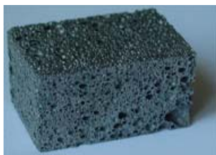
Rys. 1. Badane materiały: a) AK9/SiC z małymi pęcherzami, b) AK9/SiC, c) spieniane aluminium TiH 2 Fig. 1. Tested materials: a) AK9 / SiC in the form of small blisters, b) AK9 / SiC, c) foamed aluminium TiH 2
