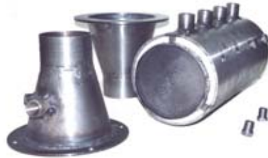
Fig. 12. Metallic enclosure of tested of catalytic converter [6]
