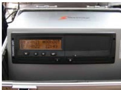
Fig. 1. View of certificated vehicles unit – digital tachograph
